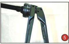
Expanding the pipe. Close levers of expanding tool, then release and rotate pipe slightly and repeat. This will ensure perfect roundness which will create a leak proof joint.
