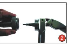
Screwing the correct size head to the expander, while lever handles are open
