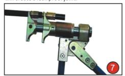
Fit Jaws of tool on joining sleeve and fitting. Close jaws.
