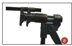
Make sure sleeve is drawn over pipe to shoulde r of fitting. Secure joint is complete
